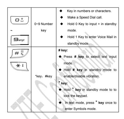
**Note**: To "press" the key in this manual means to press the key and release it. To "hold" the key means to keep pressing the key for two seconds or more.
