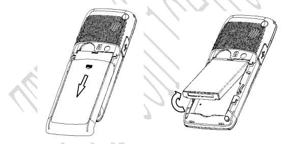
Installation: (1) Replace the battery into the battery slot, to be noted that the lower end of the battery firstly inserted. (2) Put the back-cover of the phone flatly upon the body of phone. Direct the back cover towards the locking catches on the both sides of the phone and push the back-cover of the phone upward to lock the cover into its place.
