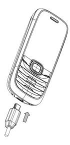
2. After the completion of charging, disconnect the charger from the phone and AC socket.
