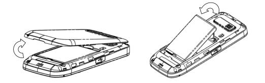
**Install**: (1) Replace the battery into the battery slot, to be noted that the lower end of the battery firstly inserted. (2) Put the back-cover of the phone flatly upon the body of phone. Direct the back cover towards the locking catches on the top/sides of the phone and slide the back cover as shown below.
