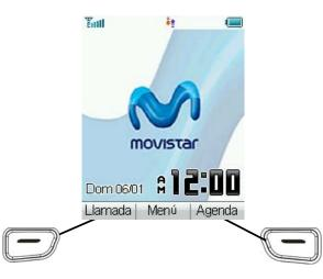
The left and right **Select Keys** are used to choose the options from the bottom of the screen.
