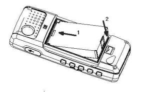
Close the case by locating the top of the plastic cover into the grooves and gently pushing the cover down to close it.
