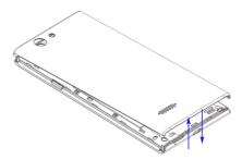
2. Hold the SIM card with the cut corner oriented as shown, and slip it into the card holder.
