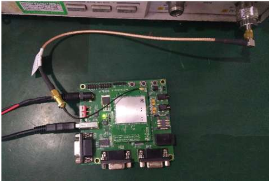
Figure 6-4 Second method to connect the module to RF test equipment
