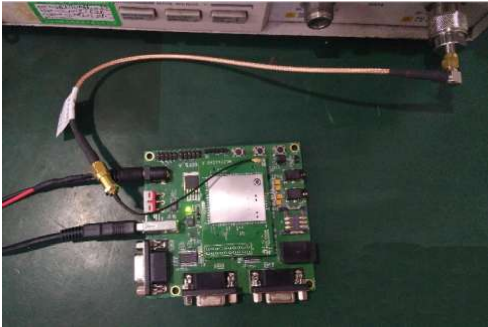
Figure 3-8 Second method to connect the module to RF test equipment
