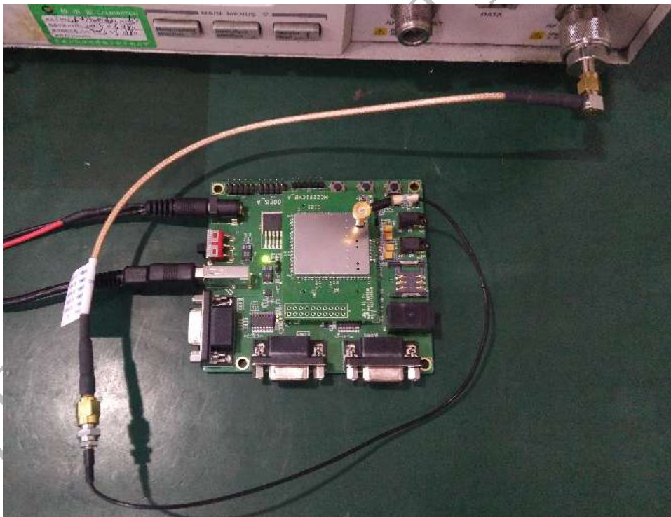
Figure 3-8 Second method to connect the module to RF test equipment
