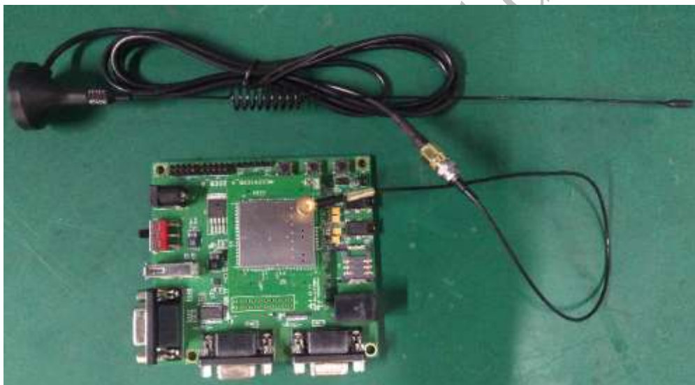
Figure 6-6 Second method to connect the module to RF antenna
