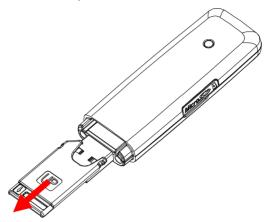
I Then insert the SIM/USIM card into the socket, here make sure that metal contact area facing to the modem.
