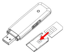
Insert the plastic socket into the modem. You can hear a click when the SIM/USIM card locks into place.
