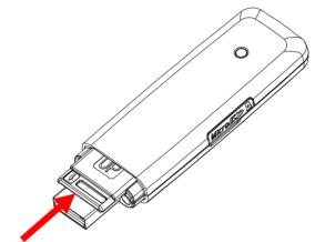
To Remove the SIM/USIM card from the USB modem
