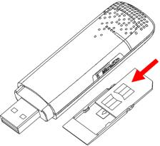
Insert the plastic socket into the modem. You can hear a click when the SIM/USIM card locks into place.
