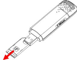
I Then insert the SIM/USIM card into the socket, here make sure that metal contact area facing to the modem.
