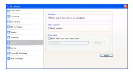
If "Start when device is available" item is selected, when user insert device into PC, the software will start running automatically.
