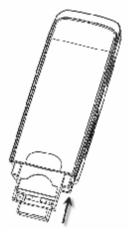
To Remove the SIM/USIM card from the USB modem,
