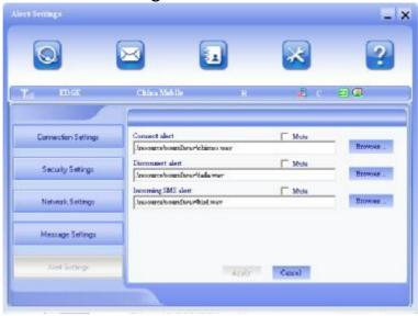
You can set "Connection alert, Disconnect alert and Incoming SMS alert" by yourself. These alerts will sound on the PC side. The audio file supports MP3、WAV、WMA and MIDI format. If you select "**Mute**", you cannot hear corresponding alert.
