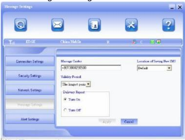
**Message Center:** Set the corresponding SMS center number the network supplier. You must input the correct SMS center number to use the SMS properly and the number will be provided by the network supplier. Please enter the country code before the number.
