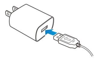
2. Insert the other end of the micro USB cable into your device's micro USB port.
