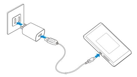
1. Insert the micro USB cable (USB plug) into the AC adapter.
