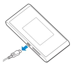
Unplug the AC adapter from the outlet, and remove the micro USB cable from the device and the AC adapter.
