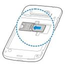
Open the microSD card holder, hold your microSD card with the metal contacts facing down and slide it in, and then close the card holder.
