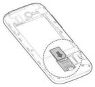
Align the connectors on the phone and the battery and slide the battery into the compartment (1). Then gently press the battery down until it is secured (2).
