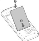
Align the back cover with the back of the phone and press the cover back into place. Make sure all the tabs are secure and there are no gaps around the cover.
