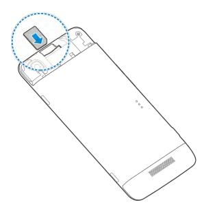
3. Replace the UICC card cover. Ensure that all the tabs are secure and there are no gaps around the cover.
