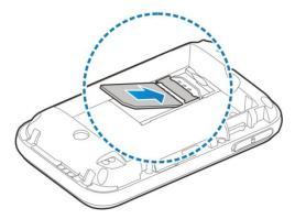
3. Insert the battery as shown with the contacts located against the metal springs, and press the battery down into the case.
