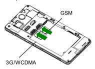
Hold your microSDHC card with the metal contacts facing down and slide it into the microSDHC card slot.
