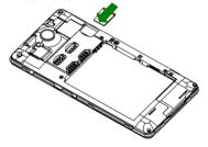
4. Align the connectors on the phone and the battery and slide the battery into the compartment. Then gently press the battery down until it is secured.
