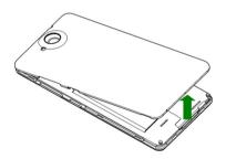
Hold the SIM card with its cut corner oriented as shown and slip it into the card holder.
