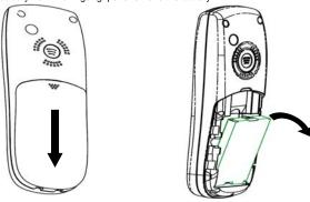
Installation: (1) Replace the battery into the battery slot, to be noted that the lower end of the battery firstly inserted. (2) Put the back-cover of the phone flatly upon the body of phone. Direct the back cover towards the locking catches on the both sides of the phone and push the back-cover of the phone upward to lock the cover into its place.
