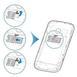
3. The microSDHC card can be installed and removed while the phone is turned on. Unmount the microSDHC card before removing it.
