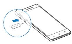
Pull out the card tray and place the nano-SIM card and the microSDXC card on the tray, as shown. Carefully slide the tray back into place.
