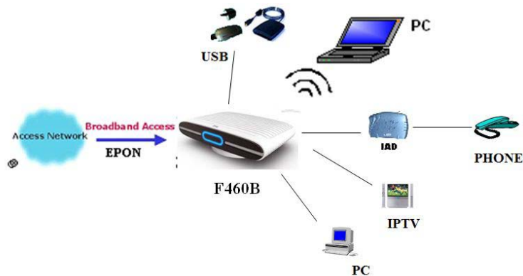
Figure 5 System Application Environment
