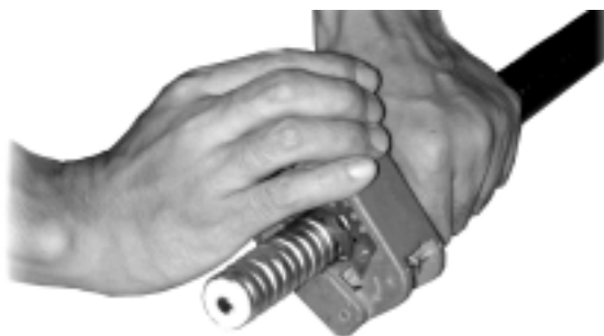
Fig. 8.6-3 Schematic Diagram of Cutting the Feeder Cable with the Cutter
