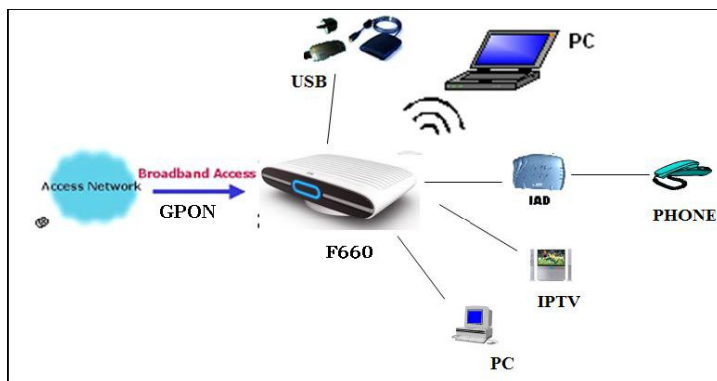
Figure 1-4 System Application Environment
