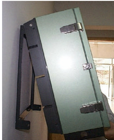
FIGURE 16 HANGING THE CHASSIS ONTO THE SUPPORT-WALL MOUNTING
