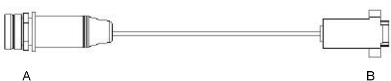
FIGURE 28 EXTERNAL MONITORING CABLE STRUCTURE
