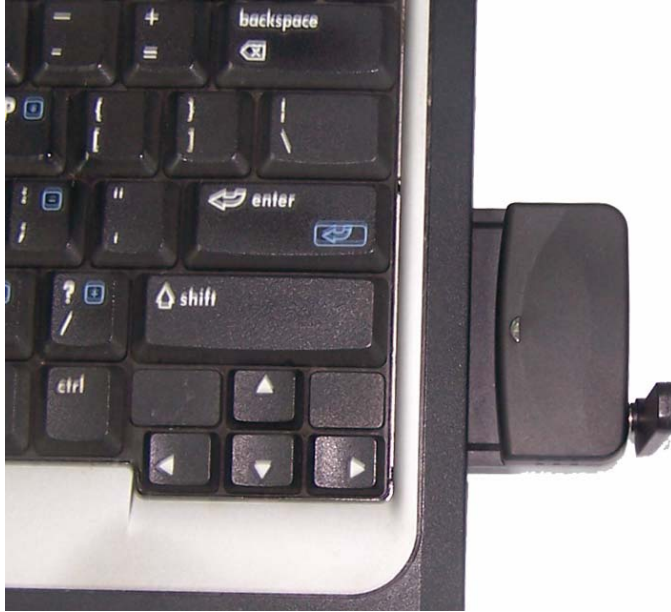
FIGURE 5 DATA CARD INSTALLATION
