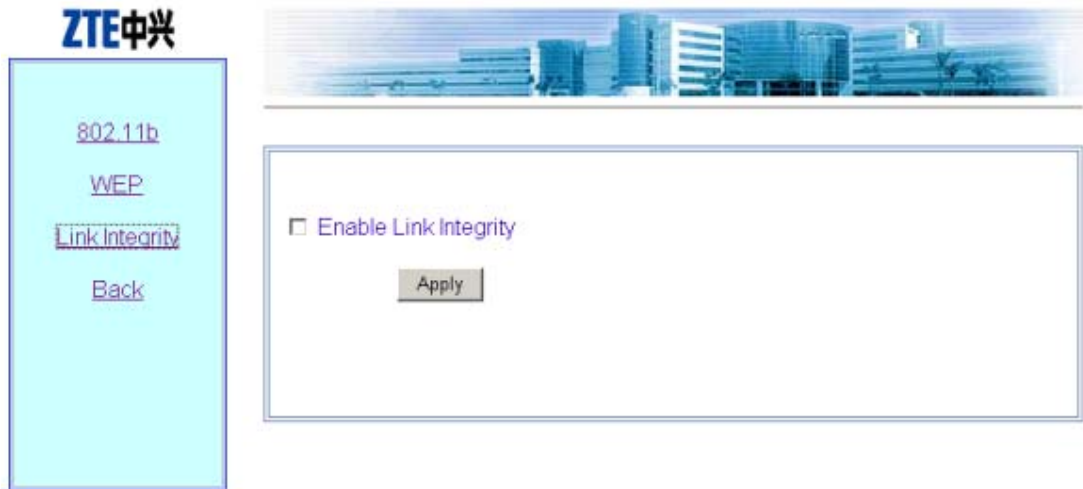
Fig. 6.4-7 Link integrity configuration page of wireless interface
