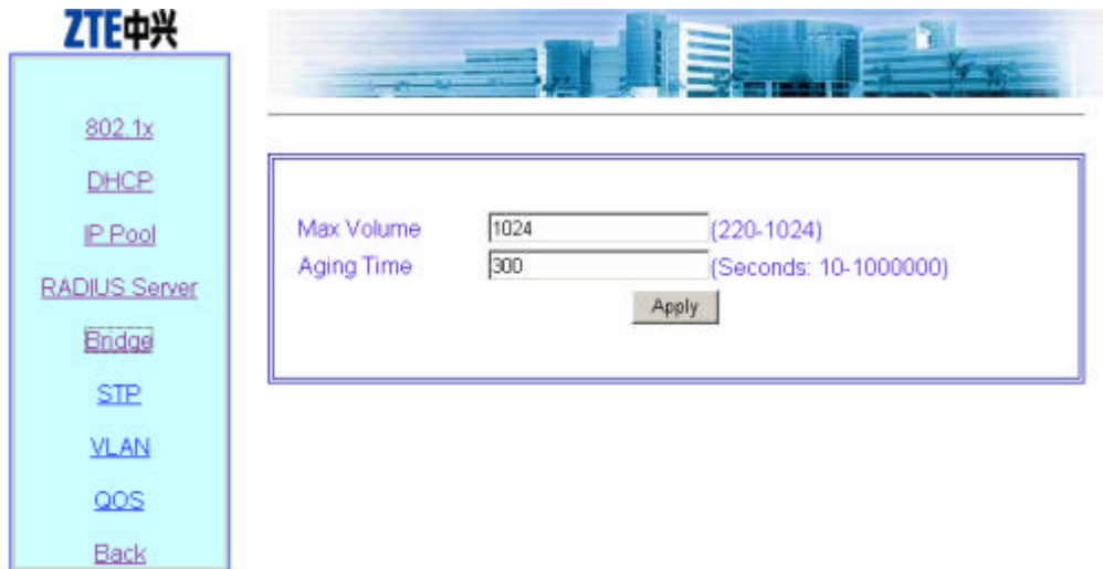
Fig. 6.3-37 Bridge Configuration Page
