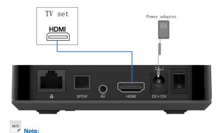
HDMI output interface simultaneously generates uncompressed high-definition video and multi-channel audio data. One HDMI data cable is capable of conveying both video and audio data.
