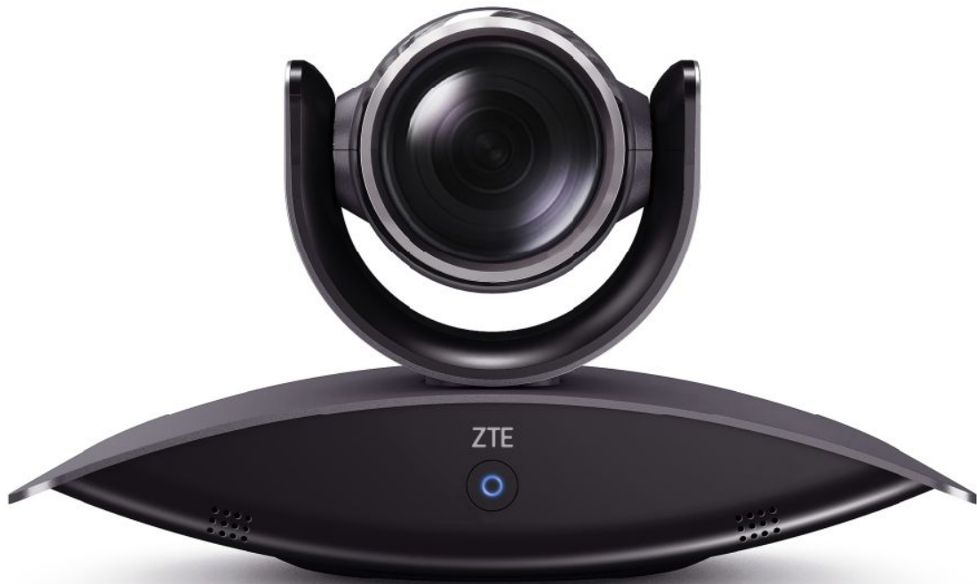
Figure 3-1 Front Panel of the ZXV10 ET501
