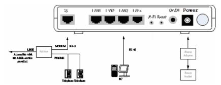
The following diagram illustrates the recommended connections and installation via WAN connector.
