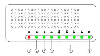
There area eight indicators on the front panel of the ZXV10 W300. These indicators indicate the service running status of the ZXV10 W300. The indicates are described in the table below.
