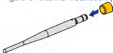
Figure 6 Antenna Installation (one)
