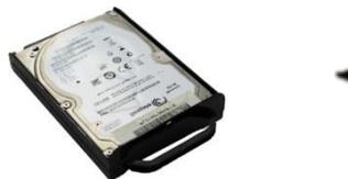
Installing a 2.5" HDD/SSD kit
