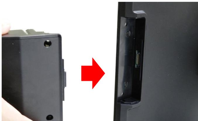
Step 4: Using two screws to secure RFID kit to the right side of the monitor.
