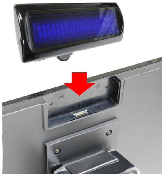
Step 4: Using two screws to secure VFD customer display to the up side of the monitor.
