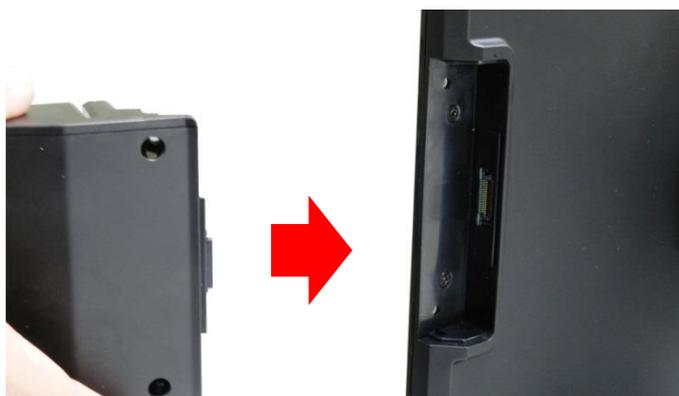
Step 4: Using two screws to secure MSR housing to the right side of the monitor.
