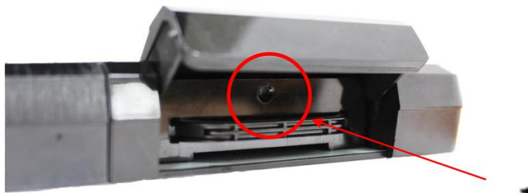
Step 5: Close the HDD cover to complete the installation.
