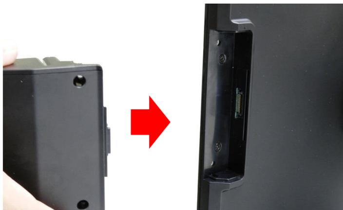
Step 4: Using two screws to secure 2-in-1 MSR housing into the right side of the monitor.
