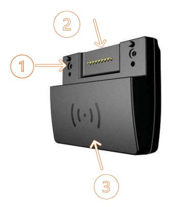
1.2.1Screw Hole: Used to fix the module and host
