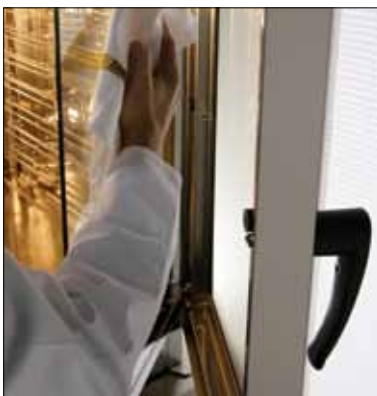
Double thermo-glazed door with drip pan to facilitate cleaning operations
