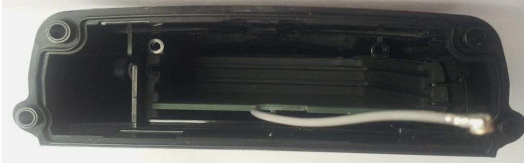
Figure 2-5 Antenna position for WLAN only WAP4 version
