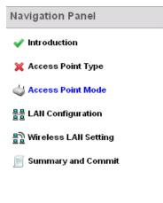
A green checkmark to the left of an item in the **Navigation Panel** defines the task as having its minimum required configuration set correctly. A red X defines a task as still requiring at least one parameter be defined correctly.
