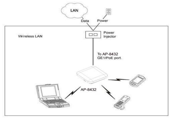
A separate Power Injector is required for each AP-8432 Access Point comprising the network.
