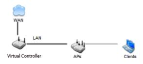
Bridge Mode - In Bridge Mode, the access point depends on an external router for routingLAN and WAN traffic. Routing is generally used on one device, whereas bridging is typically used in a larger density network. Thus, select Bridge Mode when deploying this access point with numerous peer APs supporting clients on both the 2.4 and 5GHz radio bands.
