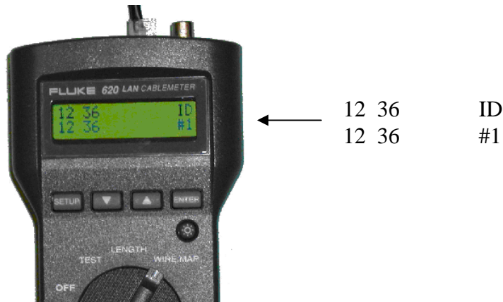
Figure 39 Correct readout when testing 2 pair cable.
