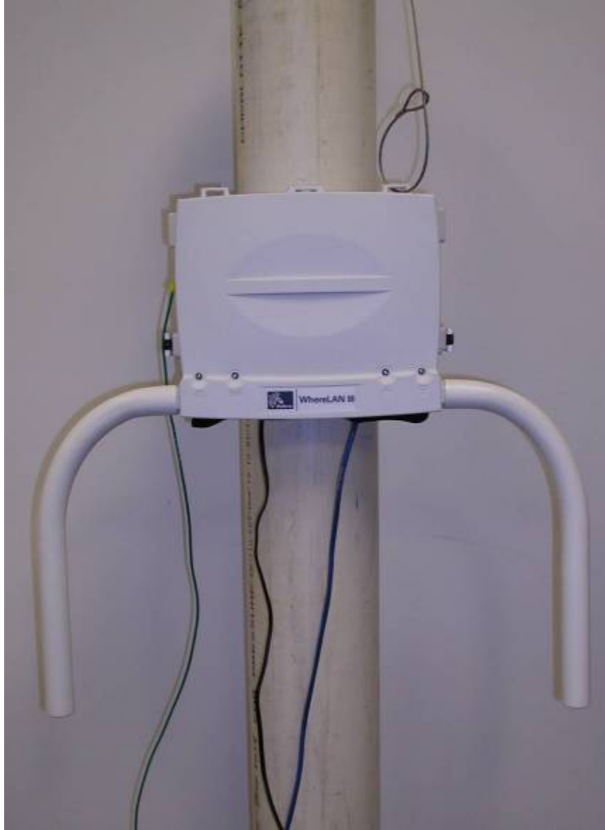
Figure 13 Location Sensor on Pole
