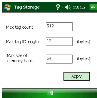
Figure 4-9 Tag Storage Window
