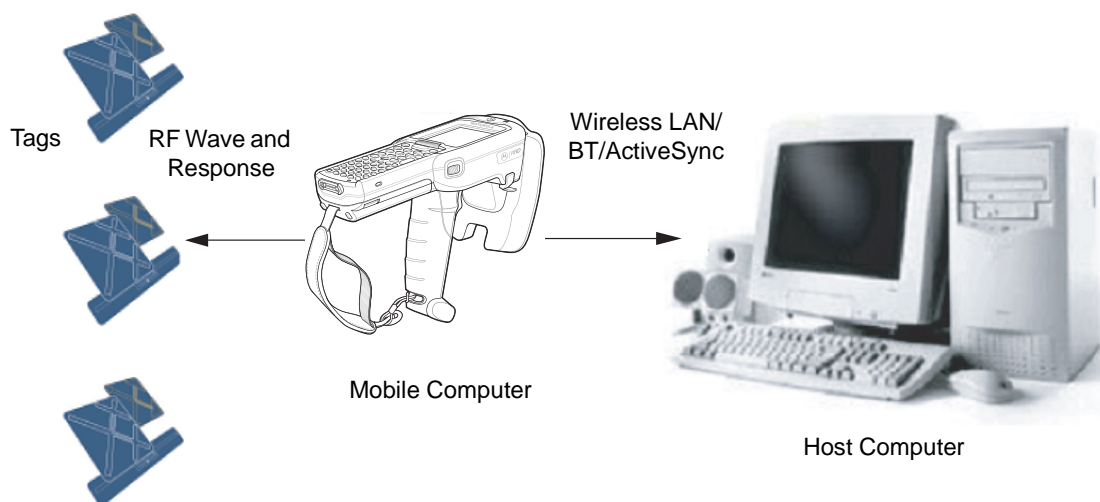
Figure 1-1 RFID System Elements
