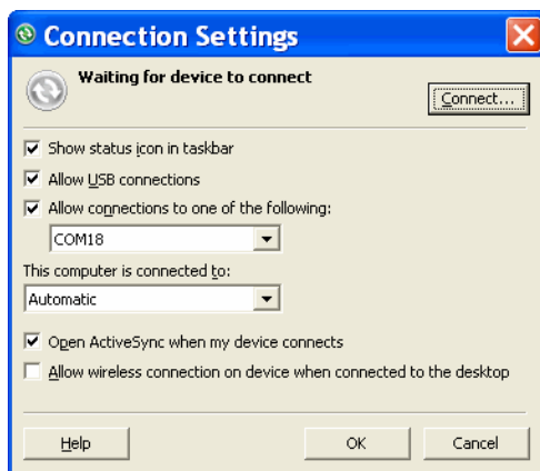
Figure 4-10 ActiveSync Connection Settings
