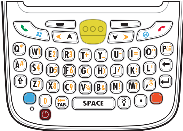
Figure B-2 QWERTY Keypad Configuration
