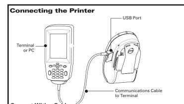
**Connect With a Cable**Refer to the Label Vista™ application on the Internet at <a href="http://www.zebra.com">http://www.zebra.com</a> for help on setting
