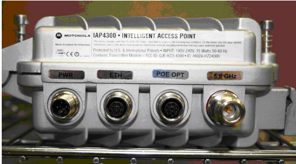
Figure 2-6 Close Up of External Connection Points
