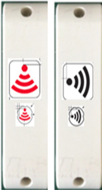
Figure 2-10 Antennae Positions of the MPACT-MB4000-01-WR and MPACT-MB4001-01-WR Beacons
