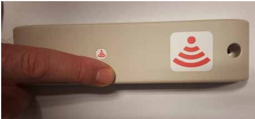
Figure 2-18 Activating Outdoor Style Beacon - MPACT-MB4000-01-WR
