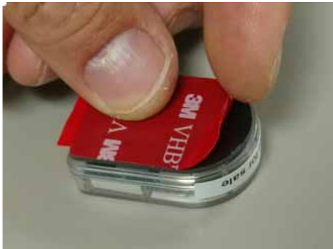
Figure 2-22 GE-MB1000-01-WR Adhesive Tape
