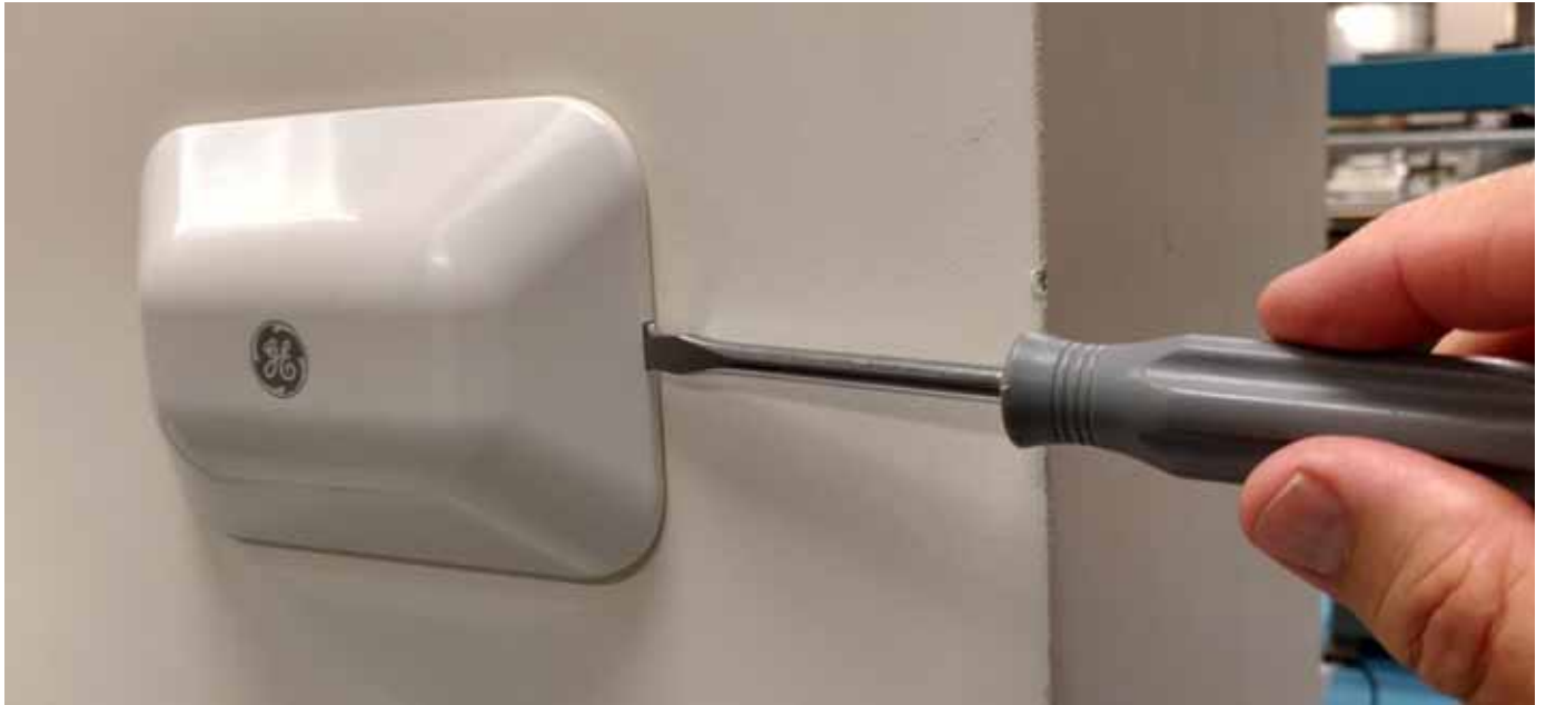
Figure 2-11 GE-MB2001-01-WR Cover and Wall Mount - Cover Removal
