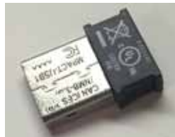
Figure 2-13 USB Style Beacon - MPACT-MB3000-01-WR
