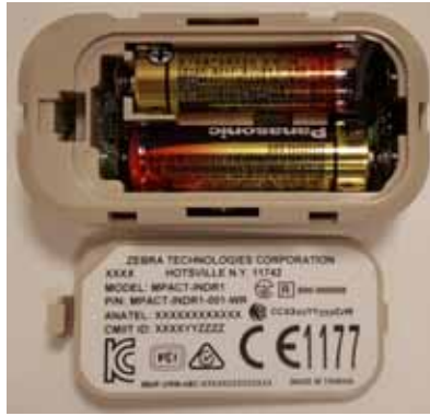
Figure 2-12 Open Battery Enclosure: MPACT-MB2000-01-WR
