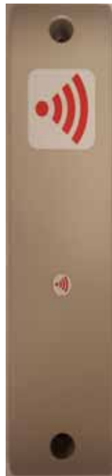
Figure 2-14 Antennae Positions for the MPACT-MB4000-01-WR Beacon
