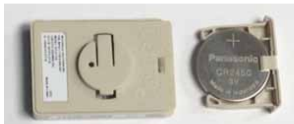
Figure 2-6 Battery Tray: MPACT-T1B20-000-WR and MPACT-T1B20-000-WR and MPACT-T1B10-000-WR
