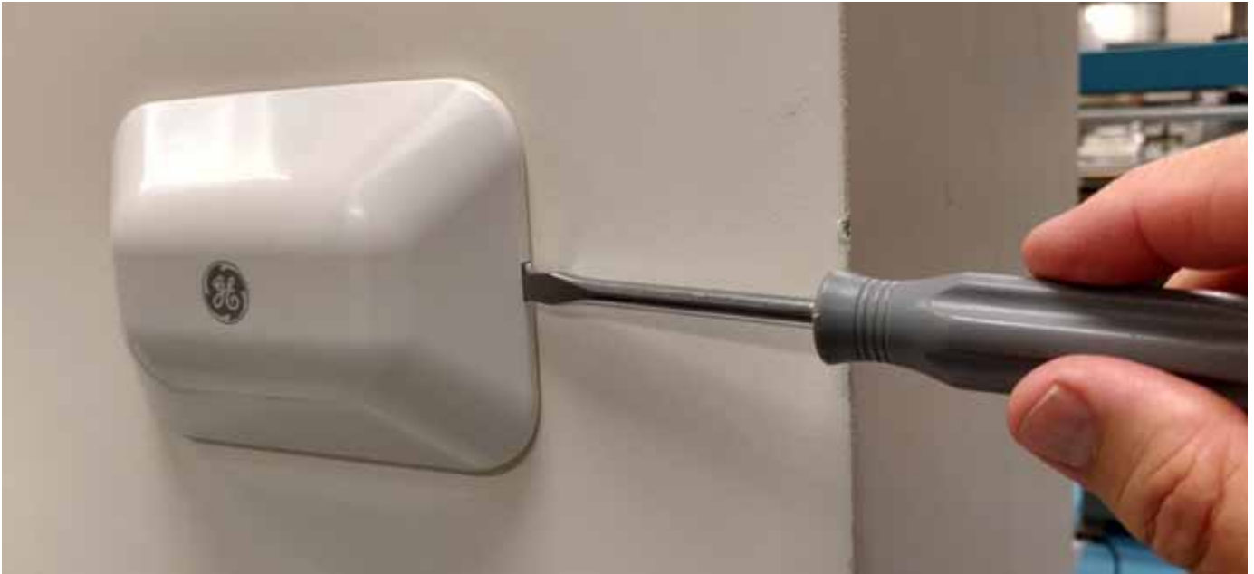
Figure 2-11 GE-MB2001-01-WR Cover and Wall Mount - Cover Removal
