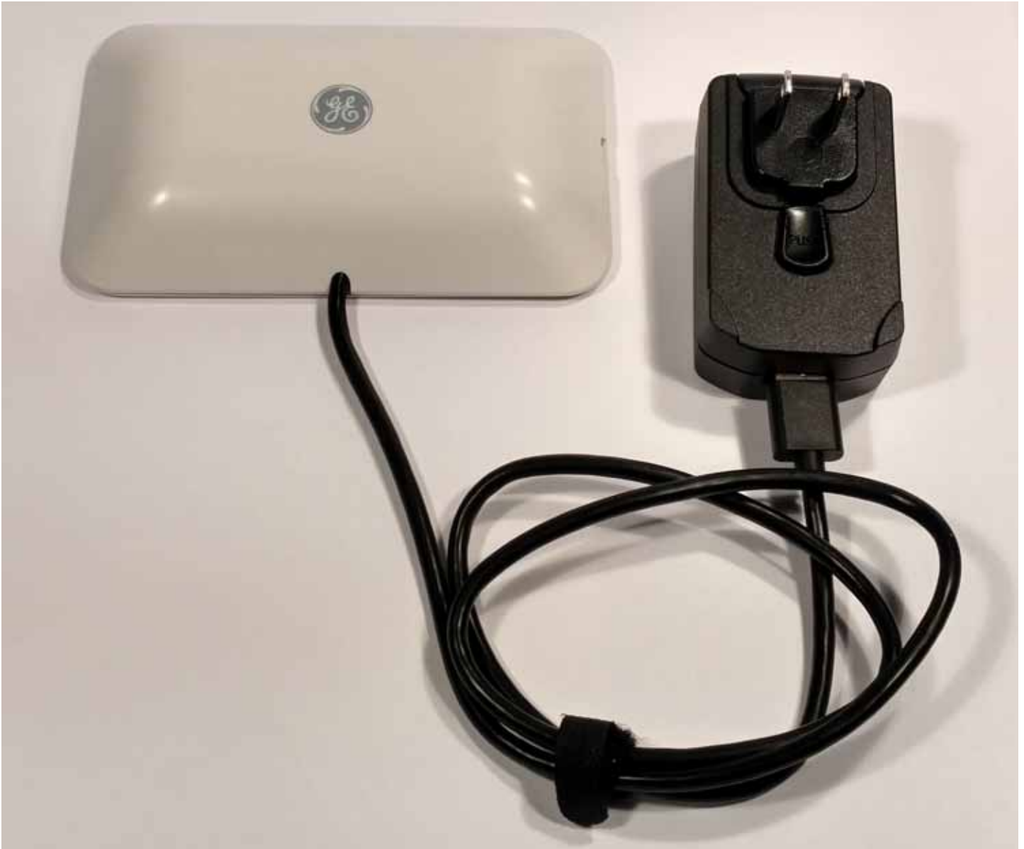
Figure 2-30 MB5000-01-WR Hub - Connect Power
