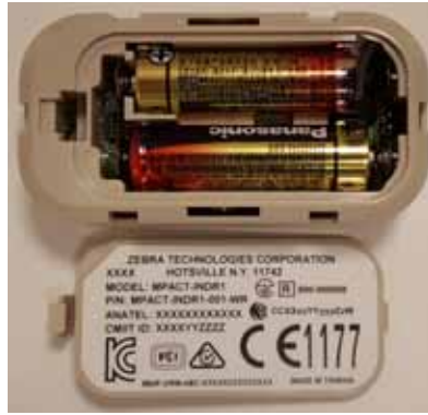
Figure 2-12 Open Battery Enclosure: MPACT-MB2000-01-WR
