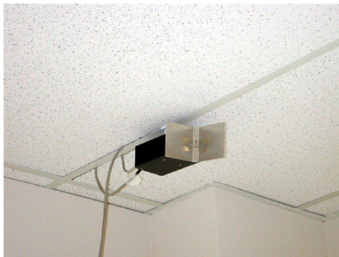
Figure 1. Typical ceiling mount for PAL-650 Receiver. Note placement of directional antenna (pointing inwards).
