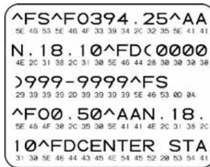
Figure 30 • Communication Diagnostics Test Printout
