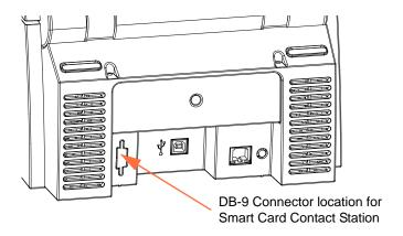
An attached external Smart Card Programmer can be used to program Smart Card chips. The following table shows the Smart Card Contact Points.
