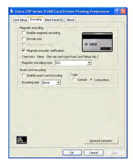
Although these options are user-selectable, they are set automatically when the Card Type is selected in the *Card Setup Tab* on page 46.
