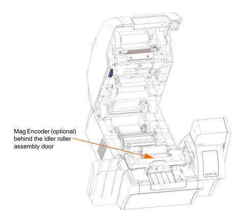
The magnetic encoder can be set for either high or low coercivity. Use the printer driver to change the encoder setting.
