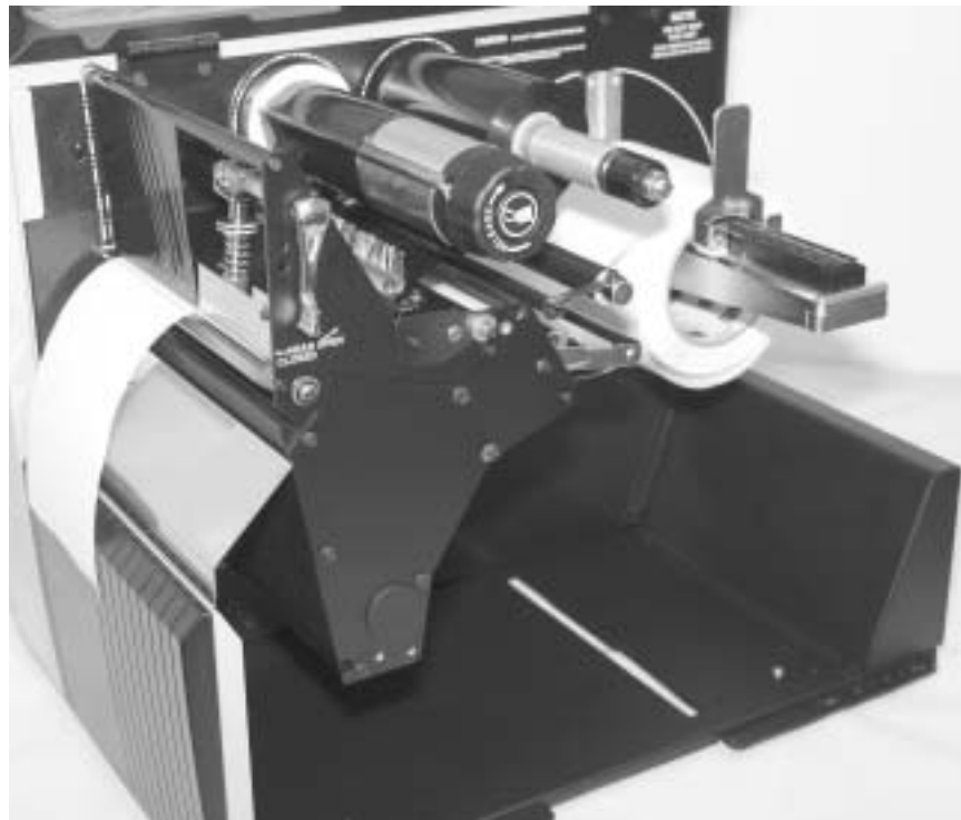
Figure 11 • Printer Loaded in Tear-Off Mode
