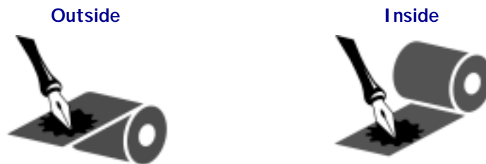
Figure 10 • Ribbon Coated on Outside or Inside
